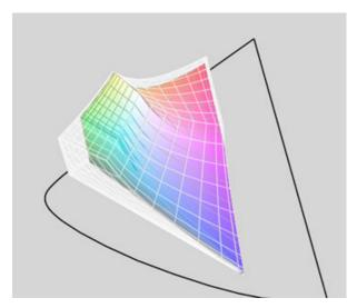
In the illustration left the large ghost diagram shows the *Adobe RGB 98* colour space, while the coloured diagram within represents the sRGB space. It's clear from this that the Adobe 98 space is bigger, and that especially in the greens and reds / oranges, some clipping if sRGB is used.
